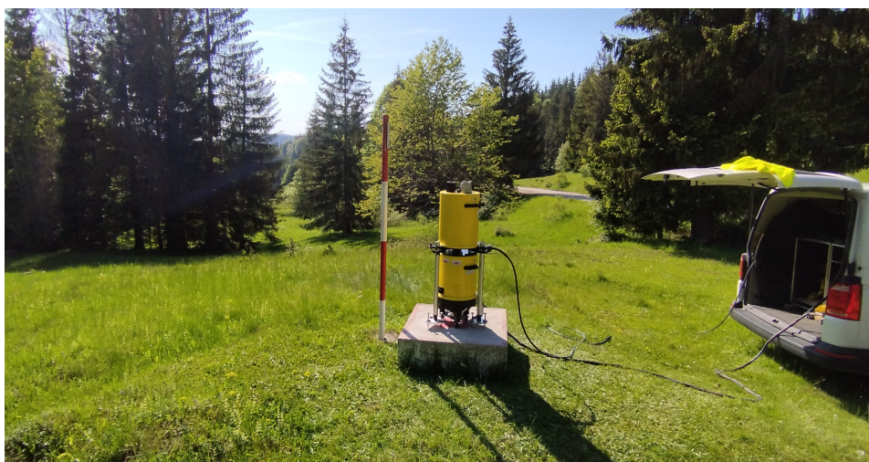
Fig. 1. Ballistic gravimeter A10 #20 during a measuring procedure on gravity control point.
